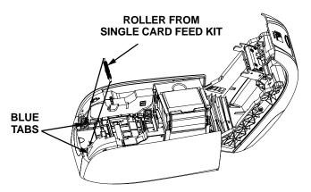
**3.** Install the black roller from the Single Card Feed Kit into the blue tabs at the front of the printer, and press roller down firmly to lock into the tabs.
